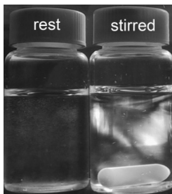
Figure 1. Picture of samples observed at rest between crossed polarizers. The samples were heated for 10 h at 80 °C, pH 2, and 2 wt % WPI. The left sample was heated at rest, and the right sample was heated while being stirred constantly.
